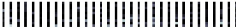
Figure 5: The 32 learned 1 \times 10 filters of the first convolutional layer of AtzoriNet [5]. Lighter color shades correspond to higher values. From bottom to top the values correspond to channels 1 to 10.
